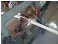
We found that by cutting various sizes of PVC tubing, both schedule 20 and 40, we could come up with several alternatives. Once you figure out the technique, wherther you rotate it into the saw blade or away from it, you can cut about 3' a minute.
